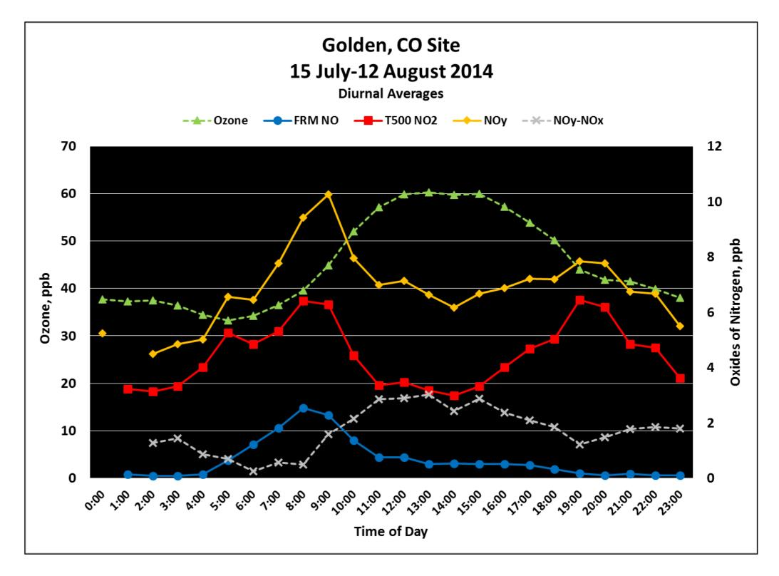
Average diurnals from EPA trace gas monitors at the Golden site (Russell Long). The  $NO_2$ -sonde has been calibrated w.r.t the combined T500-CAPS (shown above in red) and CRDS dataset. Most of the  $NO_2$ -sonde profiles were measured between 08:00-16:00 LT.
