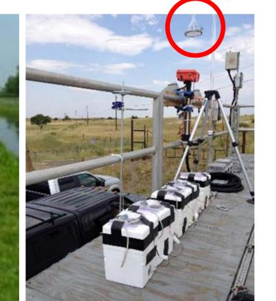
**Left:** Chemiluminescence cartoon and NO<sub>2</sub>-sonde schematic illustrating flows and key design features. **Middle:** D-AQ site map showing Golden; **Far right:** Five sondes placed on the EPA trailer roof close to the CAPS/CRDS inlet (red circle) for a side-by-side measurement at the Golden site.
