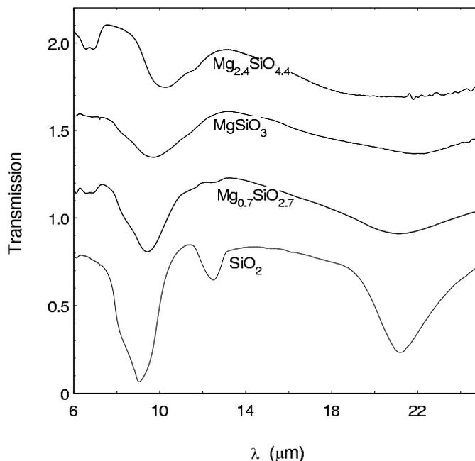
**Fig. 1.** IR transmission spectra of magnesium silicates in the binary system MgO·SiO<sub>2</sub> for various MgO/SiO<sub>2</sub> ratios. The average particle size is less than 1 μm. For the sake of clarity, the curves have been successively shifted by 0.4.
