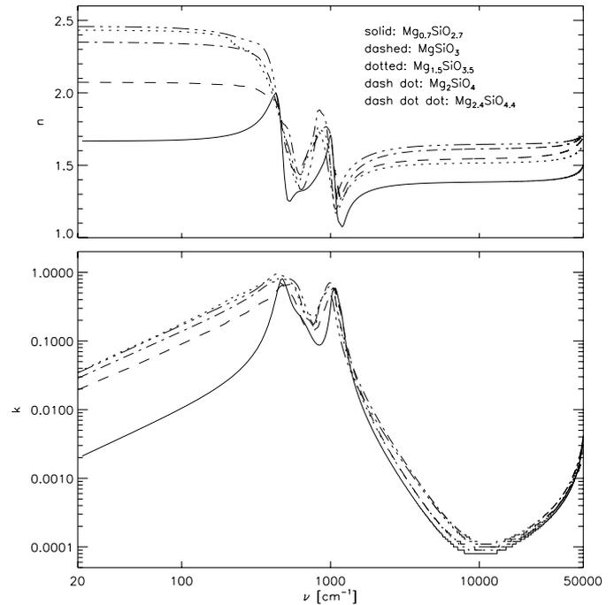
**Fig. 3.** Optical constants of amorphous magnesium silicates of varying composition derived from reflection measurements by KKR and Lorentz oscillator fit methods. The  $n$ - and  $k$ -data files can be taken from the internet homepage of the Astrophysical Institute and University Observatory Jena (<http://www.astro.uni-jena.de/Laboratory/Database/silicates.html>).
