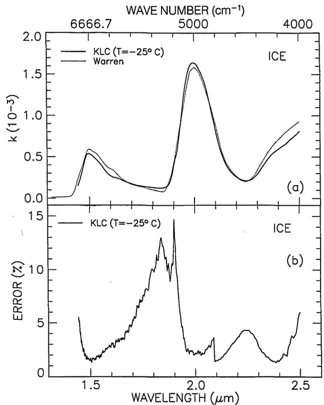
Fig. 3. (a) Imaginary part of the refractive index of polycrystalline ice at  $T = -25\text{ }^{\circ}\text{C}$  from the present measurements (KLC, solid curve) and Warren's<sup>10</sup> compilation (dashed curve). (b) Standard deviation on  $k$  for polycrystalline ice at  $T = -25\text{ }^{\circ}\text{C}$ .
