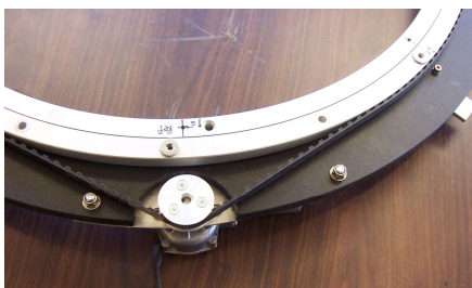
Figure 2. Bearing, drive motor and belt
