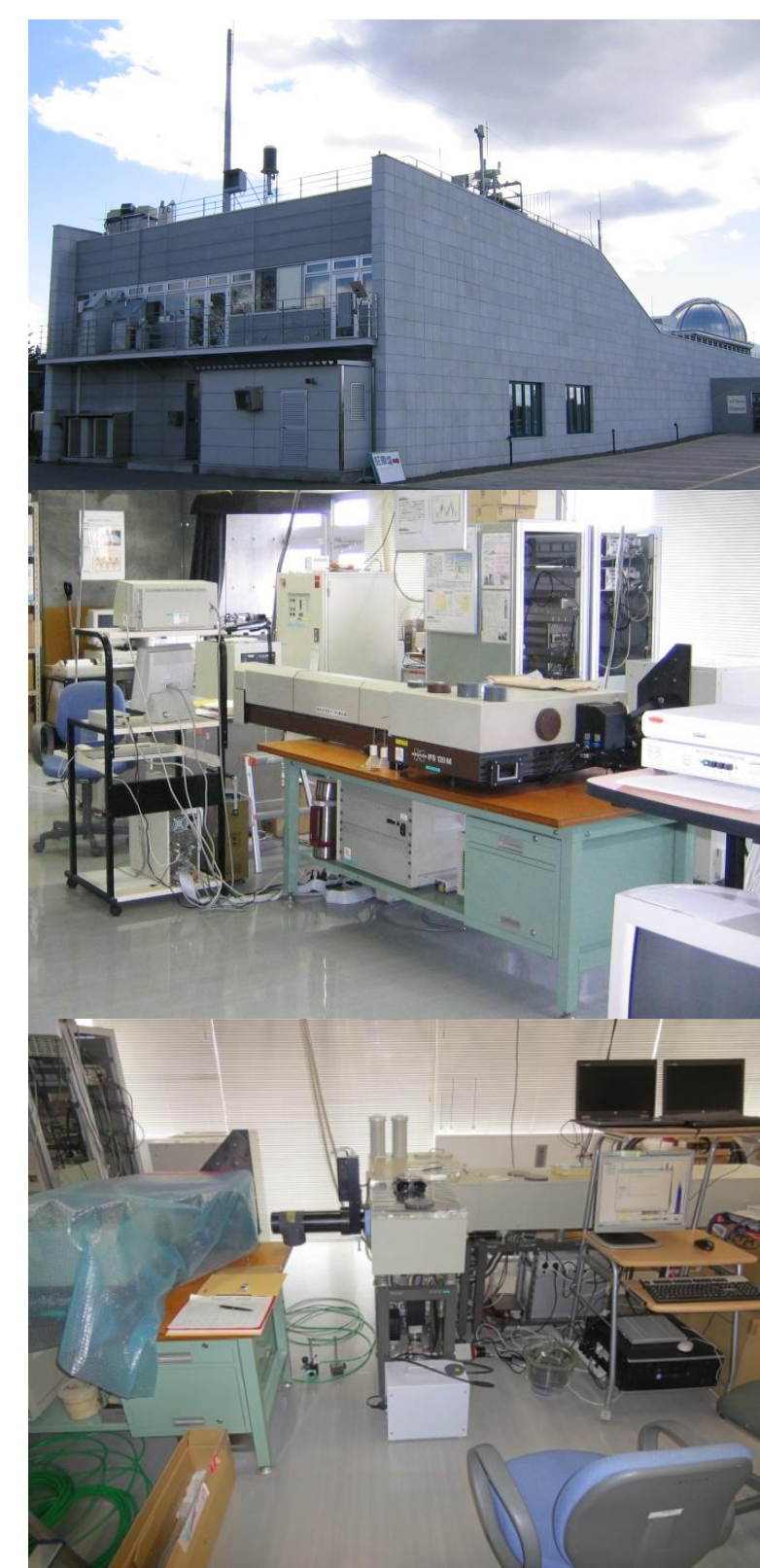
Figure 2) Rikubetsu observatory and FTIRs (middle: Bruker IFS 120M, lower: Bruker IFS 120/5 HR)
